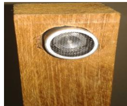
Fig.7 An ultrasonic receiver mounted in the supporting stand
